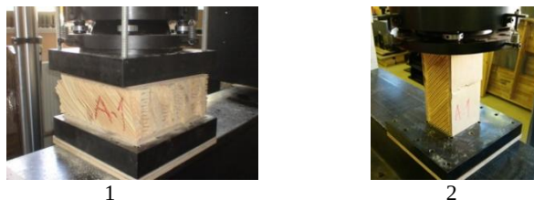
Fig. 2.5. Panel orientation in the compression testing machine:
