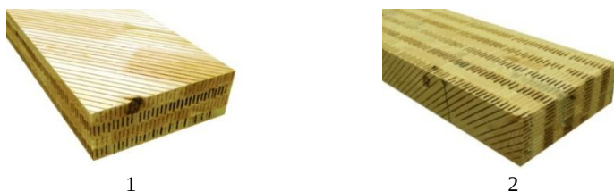
Fig. 2.3. Difference of cellular wood material orientations: 1 – parallel (KŠM 0 ); 2 – perpendicular (KŠM 90 ).
