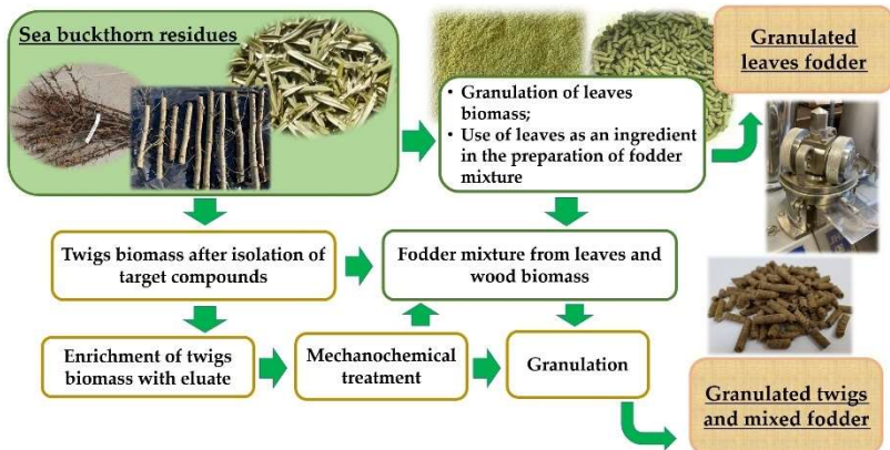
Fig.17. Scheme of sustainable processing of sea buckthorn residues to produce animal feed pellets
