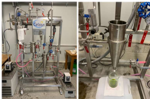
Fig. 6. Obtaining of lipophilic extracts from sea buckthorn leaves, extraction by freon
