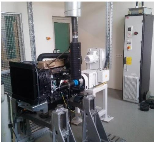
Fig. 2.4. *SIERRA CP-Engineering* engine test bench and *KOHLER KDI 1903 M* engine
