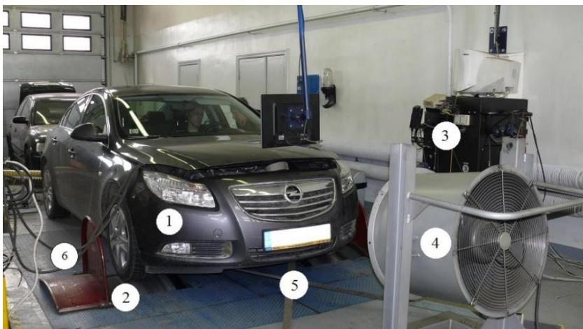
Fig. 2.3. **The tested car on the chassis dynamometer**
