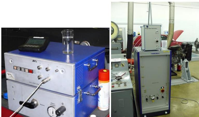
**Fig. 2.5. Fuel consumption measuring device *AVL KMA Mobile* and multicomponent exhaust gas measurement system *AVL SESAM FTIR***
