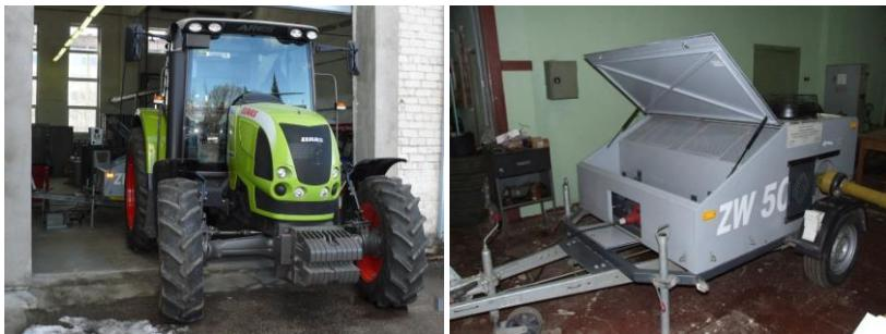
Fig. 2.2. *Claas Ares 557 ATX* tractor and **MAHA ZW500** power take-off (PTO) dynamometer
