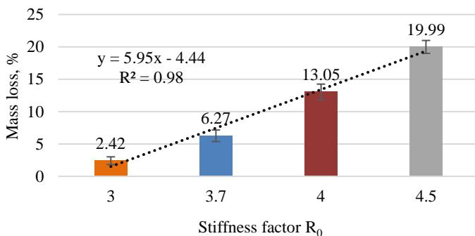
Fig. 4.3. Mass loss of hemp shive samples treated by the SE method
