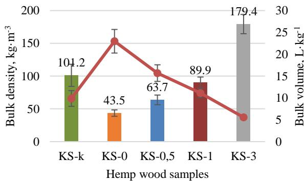
Fig. 4.4. Bulk volume (line) and bulk density (bars) for untreated and steam-explosion treated hemp shive samples
