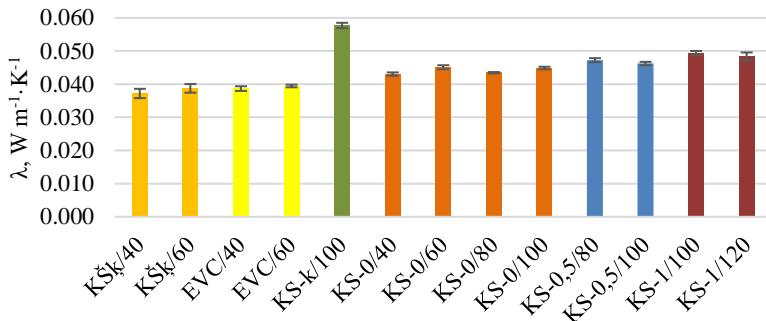
Fig. 4.7. Thermal conductivity of raw and steam-exploded hemp shive samples compared to industrial thermal insulation materials
