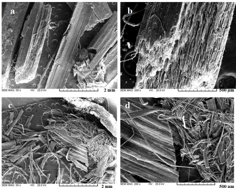
Fig. 4.5. SEM images of hemp shives before (KS-k – a and b) and after SE (KS-0 – c and d) at 50x magnification (a; c) and 200x magnification (b; d)
