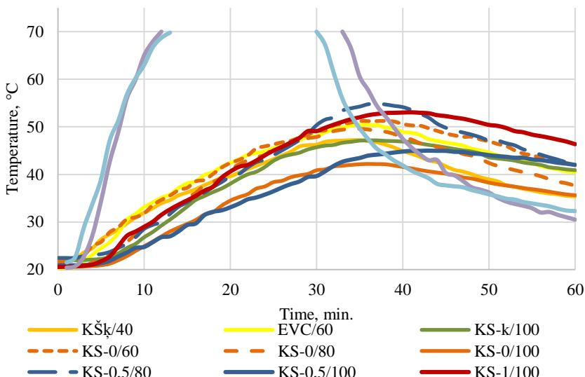
**Fig. 4.8. Thermal inertia of raw and steam-exploded hemp shive samples as compared to industrial thermal insulation materials**
