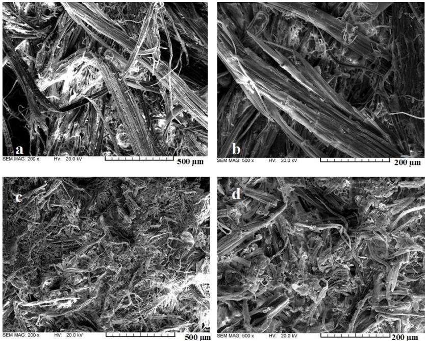
**Fig. 4.6 SEM hemp shives images after 30 seconds of (KS-0.5 – a and b) and 1 min of (KS-1 c and d) SE treatment at 200x and 500x magnifications.**
