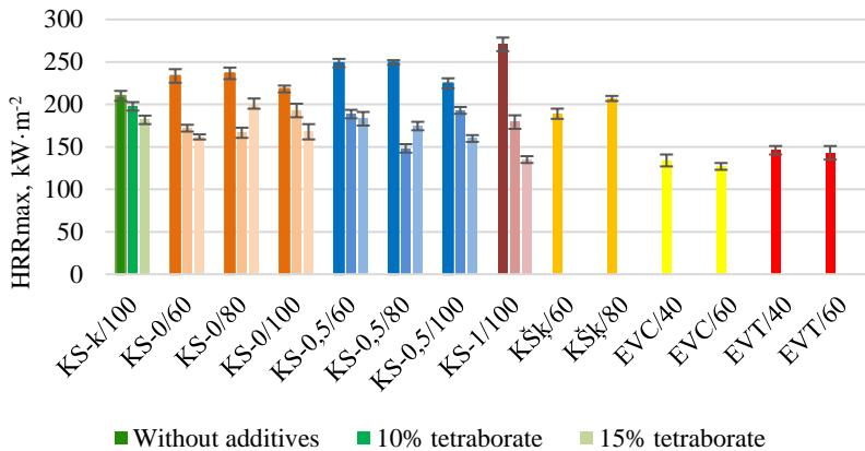
**Fig. 4.11. Maximum burning capacity ( $HRR_{max}$ ) per unit area for untreated and steam-explosion hemp shive samples with 10 and 15% fire retardant additive**
