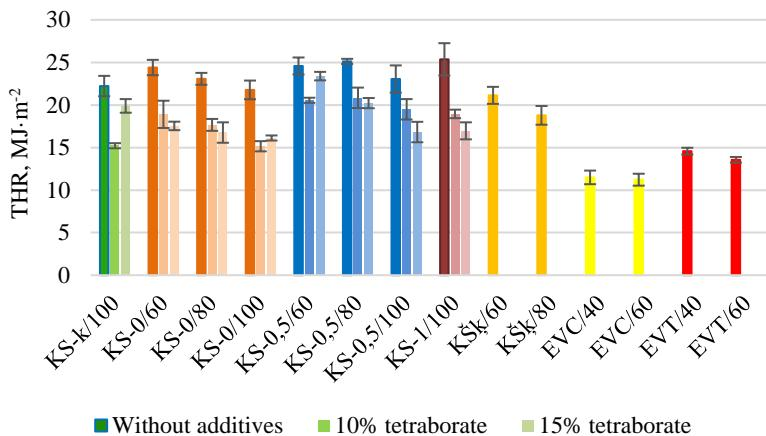
**Fig. 4.10. Total heat release (THR) per unit area in 300 seconds for untreated and steam-exploded hemp shive samples with 10 and 15% fire retardant additive**
