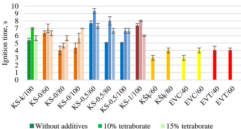
**Fig. 4.9. Ignition time of untreated and steam-explosion treated hemp straw shives at different densities**
