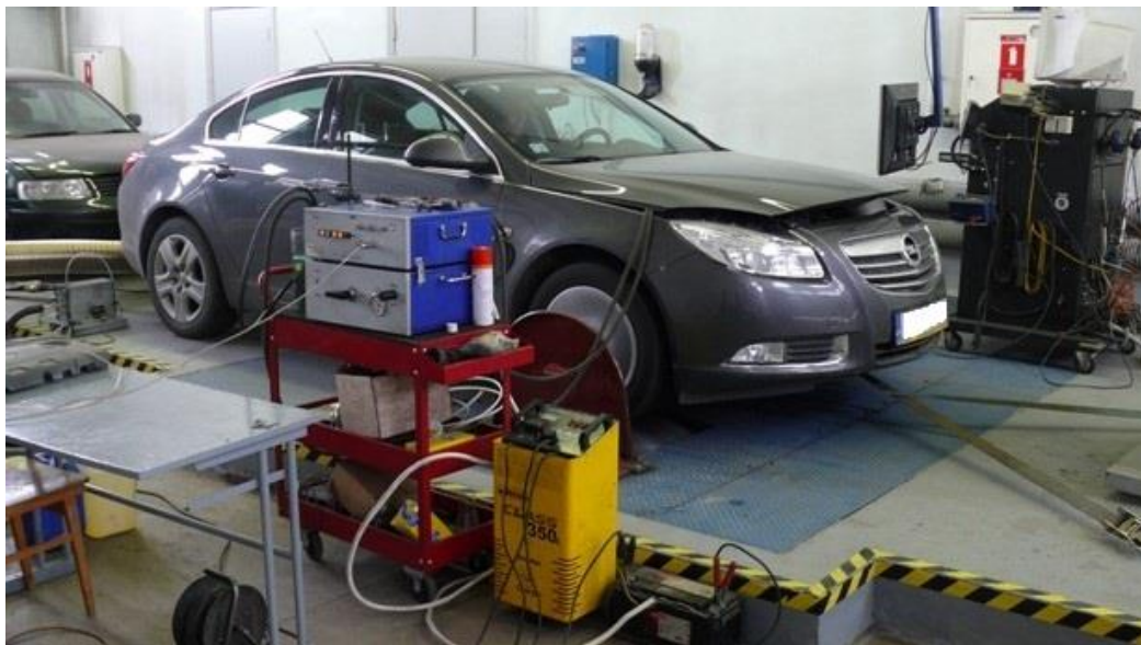
Fig. 1. Tested car on the chassis dynamometer
