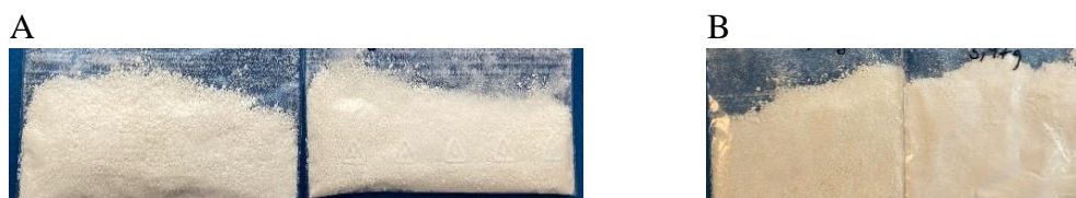
Fig. 3.11. Dehydrated sauerkraut juice on a vertical spray-dryer; (A) samples dried with starch solution and (B) starch solution and maltodextrin additive /
