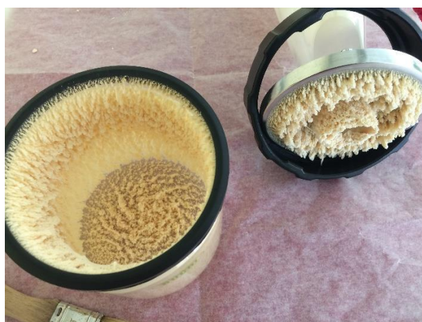
Fig. 2.8. Vertically spray-dried sauerkraut juice with maltodextrin
