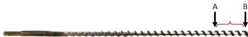
Figure 3.21. Extrudate formation sections
