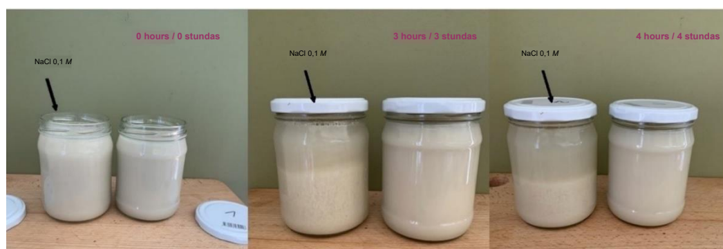
Figure 3.2. Visual observation of oat protein aggregation immediately after preparation and incubation for 3 and 4 hours at 75 °C /
