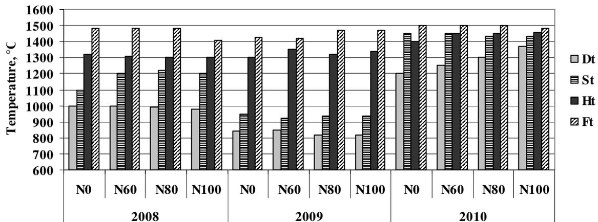
Fig. 3. Ash melting behaviour oxidizing atmosphere depending on the linseed variety “Scorpion” growing year, and N fertilizer rates: Dt – deformation temperature, St – sphere temperature, Ht – hemisphere temperature, Ft – flow temperature
