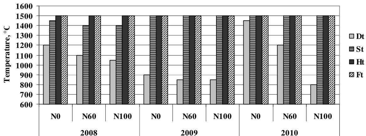
Fig. 2. Ash melting behaviour oxidizing atmosphere depending on the local hemp “Pūriņi” growing year, and N fertilizer rates: Dt – deformation temperature, St – sphere temperature, Ht – hemisphere temperature, Ft – flow temperature
