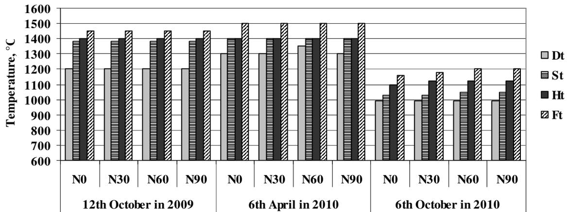
Fig. 1. Ash melting behaviour oxidizing atmosphere depending on the reed canary grass variety “Marathon” harvesting time, and N fertilizer rates: Dt – deformation temperature, St – sphere temperature, Ht – hemisphere temperature, Ft – flow temperature
