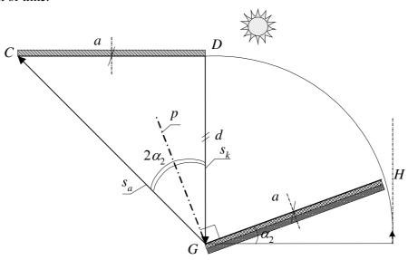
Fig. 3. Detection scheme for right mirror rotation angle  $\alpha_2$
