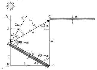
Fig. 2. Detection scheme for left mirror rotation angle  $\alpha_I$
