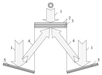
Fig. 1. **Principal scheme of solar collector with reflectors:** 1 – falling sun rays, 2 – collector cover (glass), 3 – absorber, 4 – reflection sun rays, 5 – reflectors
