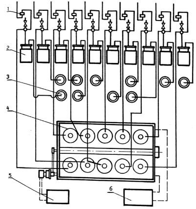
Fig. 1. Unit for anaerobic fermentation of biomass: 1 – pressure gauge, 2 – gas cylinder, 3 – receptacle for liquid, 4 – container with bio-reactors, 5 – automatic mixing unit, 6 – automatic temperature maintenance unit
