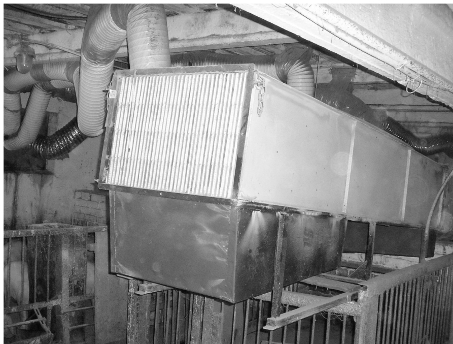
Fig. 2. Experimental heat exchanger testing in the fattening pig barn with 500 animal places
