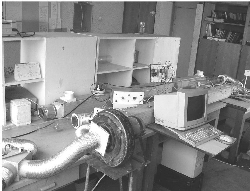
Fig. 1. Heat exchanger model test in the laboratory
