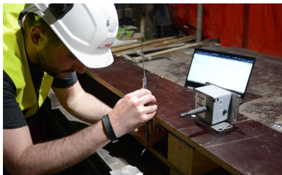
Figure 3 Adjustment of deflection using iron plates and a vernier caliper
