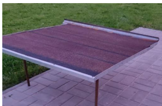
Figure 2. The rainwater harvesting system from the roof with bituminous tiles.
