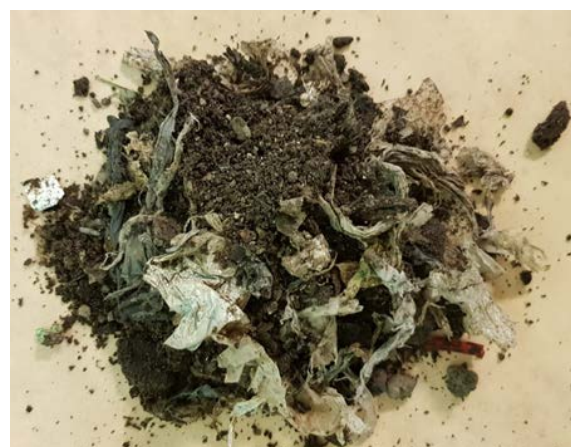
Figure 3. Composition of the biocover (20% soil, 20% compost and 60% fine fraction of waste).
