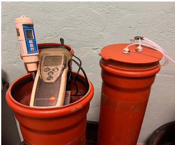
Figure 5. Performing measurements for experimental tubes. The humidity and temperature of biocover are determined. The results obtained are given to a measuring device that determines the amount of emissions. In parallel, emissions measurement is carried out.
