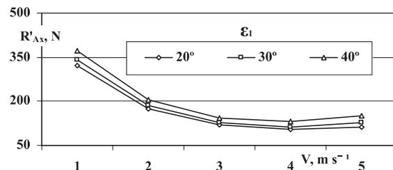
Figure 4. Draft resistance of the lifting surface caused by soil adhesion depending on the initial lifting angle  $\epsilon_1$  and speed  $v$ .
