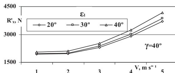
Figure 5. Total draft resistance of the lifting surface caused by soil gravity, inertia forces and adhesion depending on the initial lifting angle  $\epsilon_1$  and speed  $v$ .
