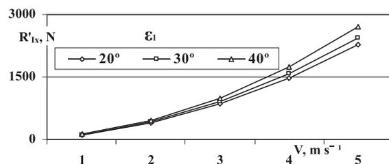
Figure 3. Draft resistance of the lifting surface caused by the soil inertia forces of the soil strip depending on the initial lifting angle  $\epsilon_1$  and speed  $v$ .
