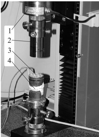
Fig. 4. Device for measuring horizontal stress:
