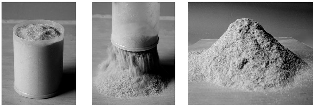
Fig. 2. Obtaining of the angle of repose.
