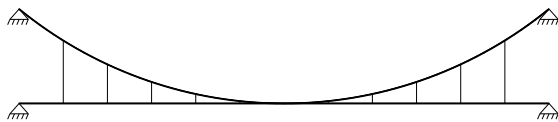
Figure 4. Suspension bridge stabilization by connecting of main cable and girder at the centre of the span
