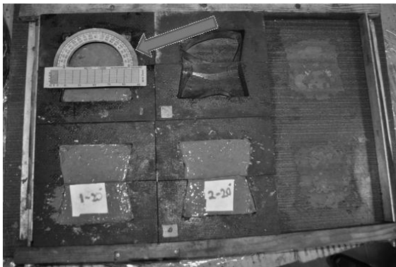
Figure 3. Samples view for pull-out tests. Is shown how were oriented single fibers in the concrete matrix corresponding to future stretching direction
