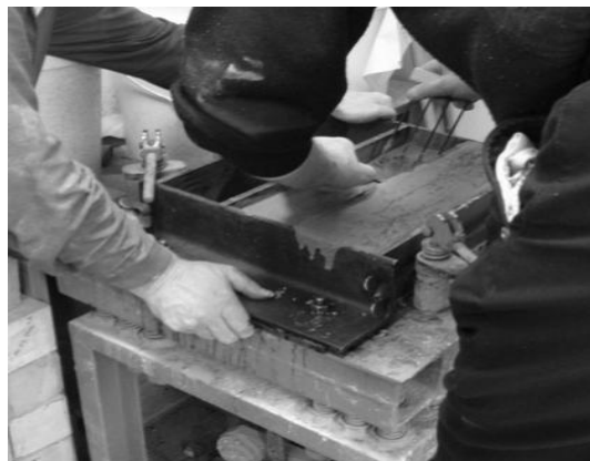
Figure 2. Combing fibers on the vibrating table
