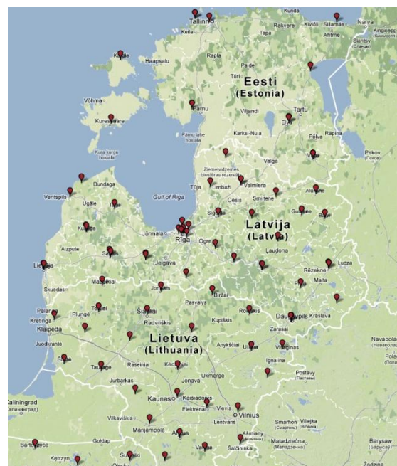
Figure 1. EUPOS ® reference station subnetwork in the Baltic countries including LatPos and EUPOS ® -Riga
