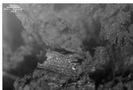
Figure 4. Micrograph of pores for samples which are made by plant fillers burning method
