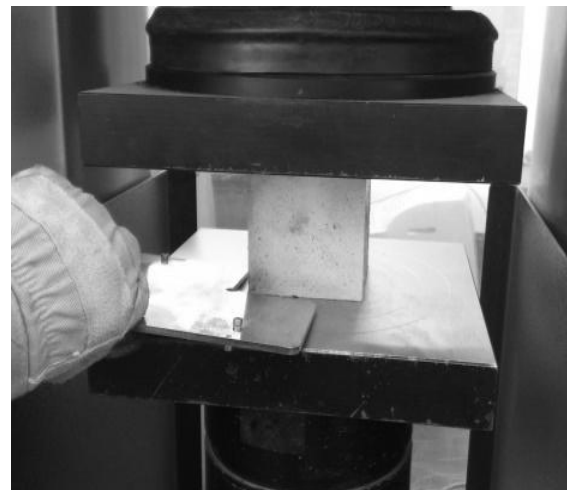
Figure 1. The sample is centered in the testing machine for compression test
