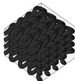
Figure 1. Structure of weft knitted fabric laminate (created in WeftKnit software (KU Leuven))
