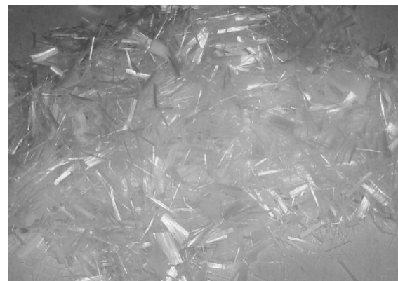
Figure 9. Polymeric micro synthetic fibers (fiber length \approx 5-6 mm, diameter \approx 1mm)
