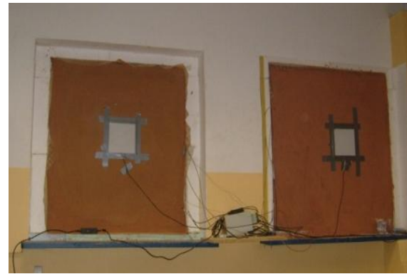
Figure 5. Heat flow plates to measure the heat transmittance and thermocouples to measure the temperature of surfaces of the wall
