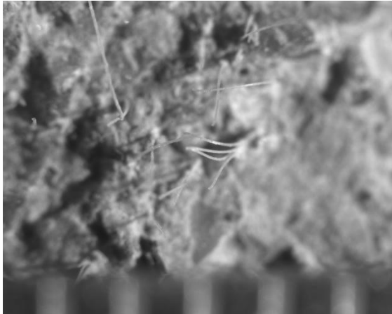
Figure 18. Micro synthetic fibers on a macro-crack surface
