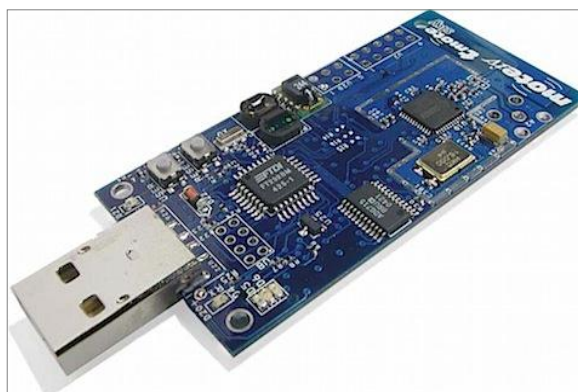
Fig. 1. Tmote Sky with on-board light and humidity sensors
