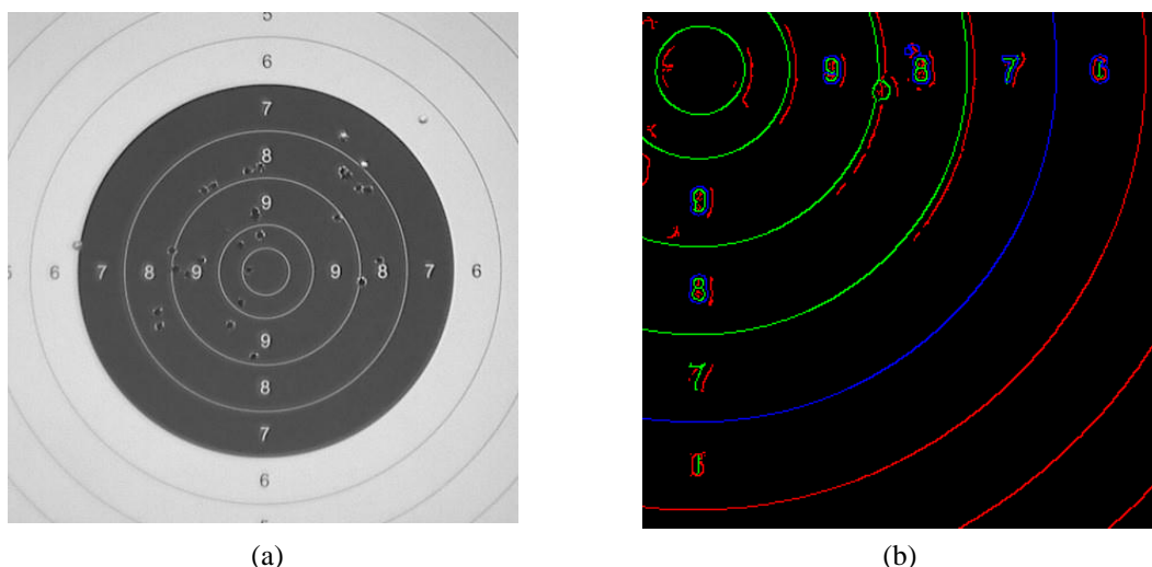
Fig. 4. (a) An image of the shooting target. (b) Ridges (green), edges (blue) and valleys (red) of the target fragment.
