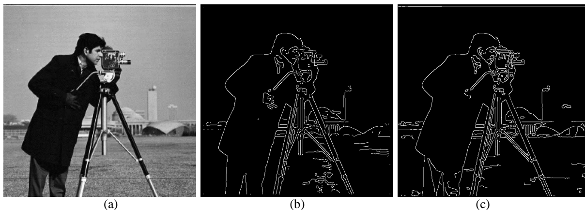
Fig. 3. The original image (a), edges detected with Canny algorithm (b) and the proposed algorithm (c).
