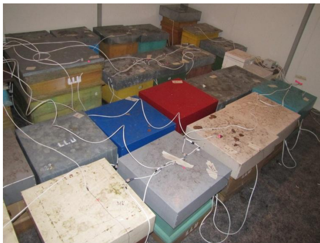
Fig. 5. Developed bee hive temperature measurement system in wintering building
