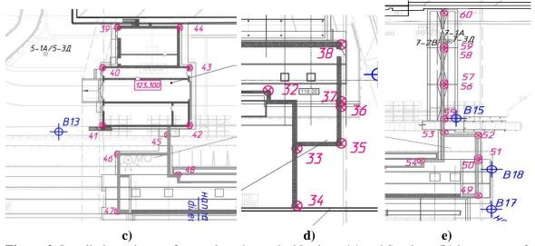
**Figure 3.** Installation scheme of control marks on the Northern (a) and Southern (b) basements of the NSC Service Zone, settlement deformation marks on the southwestern end wall (c) Arches of the NSC (marks 39 - 48), settlement deformation marks on the north-eastern (d) (marks 32 - 38) and south-eastern (e) (marks 49 - 60) end walls of the Arch of the NSC
