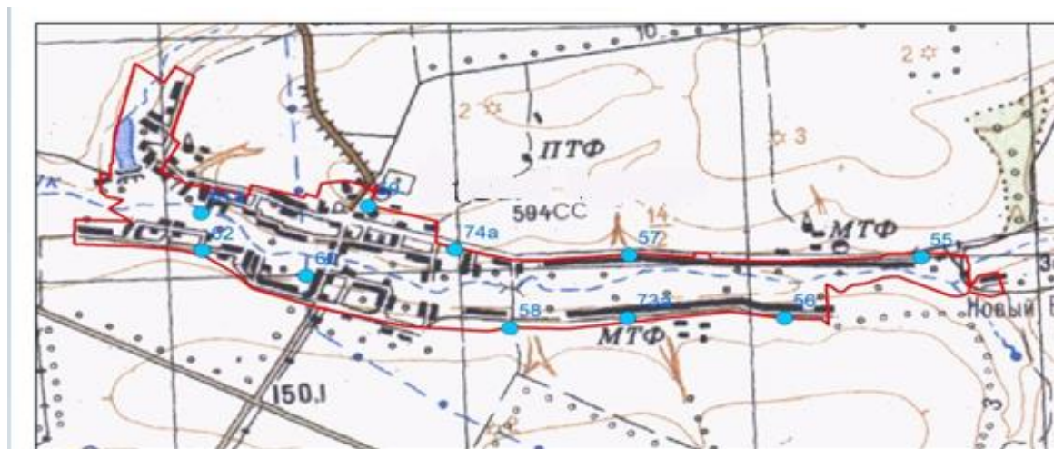
Fig. 4. Scheme of the plan basis with points of geodetic network
