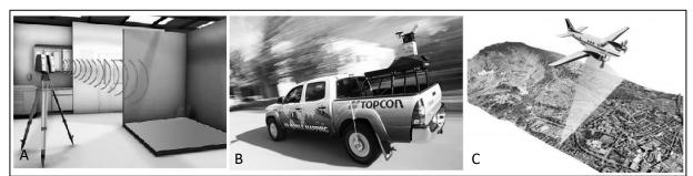
Fig, 1. Methods of laser scanning: A) static laser scanning in room on a tripod [16]; B) mobile laser scanning outside from the car [17]; C) aerial laser scanning from an aircraft [15]
